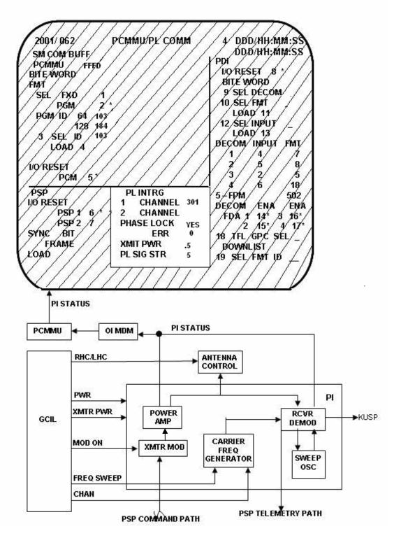
Figure 3-1. Payload interrogator
