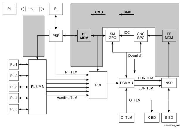
Figure 1-2. Payload telemetry overview
