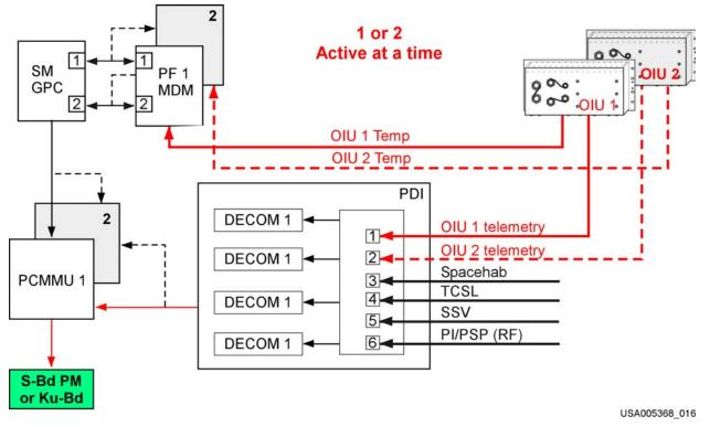
Figure 8-6. Telemetry Path
