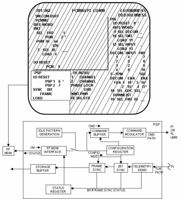
Figure 2-1. Payload signal processor
